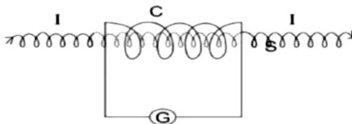
Current  $I$  through the solenoid  $S$  changes from  $2\ A$  in one direction to  $-2\ A$  in the opposite direction within an interval of  $2\ s$ .
