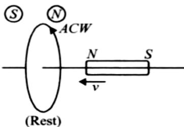
(Coil face behaves as North pole to oppose the motion of magnet.)
