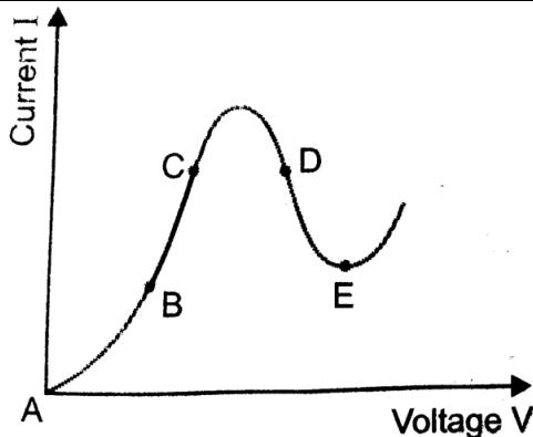
Graph showing the variation of current versus voltage for a material GaAs as shown in figure. Identify the region of
