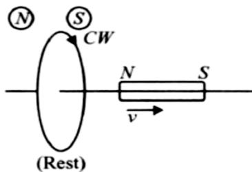
(Coil face behaves as South pole to oppose the motion of magnet.)
