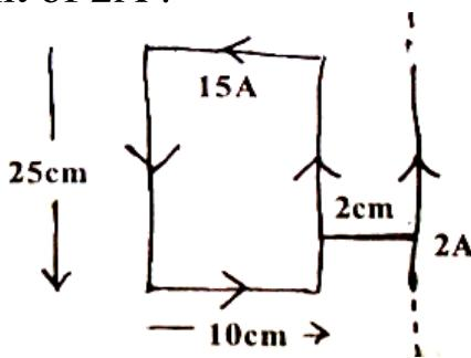
What is the direction and magnitude of the net force acting on the loop ?  $3 + 2 = 5$
