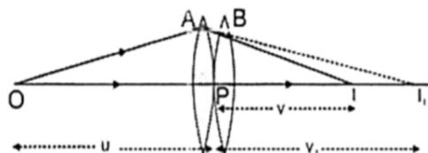
Two thin lenses, of focal length  $f_1$  and  $f_2$  are kept in contact. Let O be the position of the object and let  $u$  be the object distance. The distance of the image (which is at  $I_1$ ), for the first lens is  $v_1$ .
