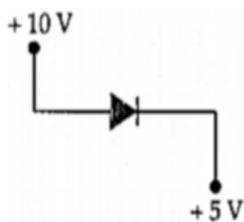
Explanation: The p-side is at higher potential (+10V) and n-side is at lower potential (+5V).
