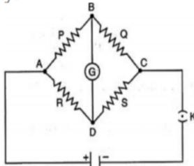
Galvanometer G is connected between points B and D and battery B is connected between A and C. Now in the balance condition, when the deflection in the galvanometer is zero in the closed mesh ABDA, then by applying Kirchhoff's law,
