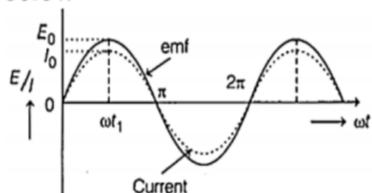
(d) Phasor diagram is as shown in figure below
