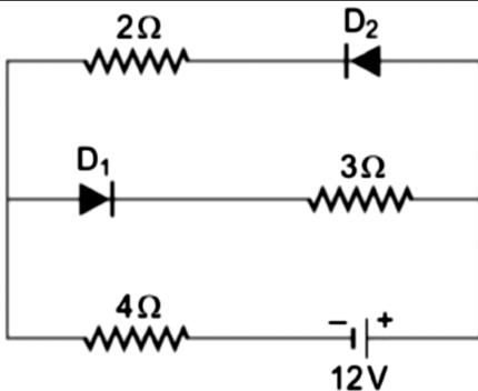
Find the current flowing through each diode in the circuit.
