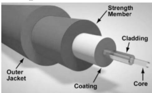
An optical fibre is a thin rod of high-quality glass. Light/infrared getting in at one end undergoes repeated total internal reflection and emerges at the other end. Optical Fibre is wave guided die – electric cable which non-conducting in nature used to data transmission using light pulses travelling in it. It transmits the light without any loss of energy. From one place to another for longer as well as for a shorter distance.
