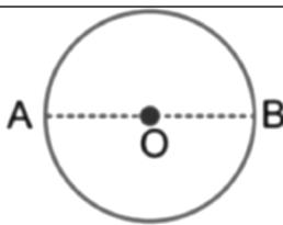
A wire of resistance  $12\Omega/m$  is bent to form a complete circle of radius 10 cm. The resistance between its two diametrically opposite points A & B as shown in figure is
