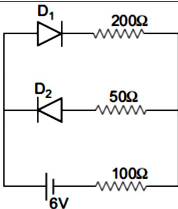
Diode  $D_1$  offers a resistance of  $50\Omega$  and  $D_2$  an infinite resistance. It means diode  $D_1$  conducts and diode  $D_2$  does not conduct. So for conducting path through diodes,
