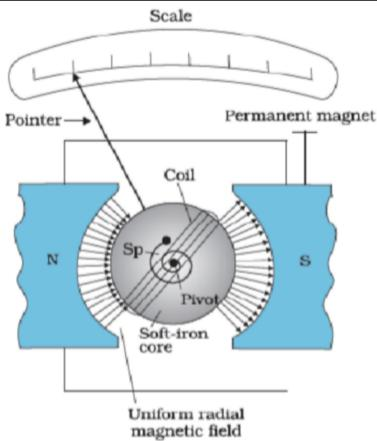
The galvanometer is a device used to detect the current flowing in a circuit or a small potential difference applied to it. It consists of a coil with many turns, free to rotate about a fixed axis, in a uniform radial magnetic field formed by using concave pole pieces of a magnet. When a current flows through the coil, a torque acts on it.
