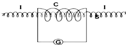
Current  $I$  through the solenoid  $S$  changes from 2 A in one direction to 2 A in the opposite direction within
