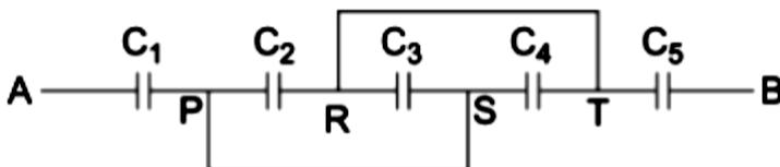
(ii) Capacitors  $C_2$ ,  $C_3$  and  $C_4$  are in parallel
