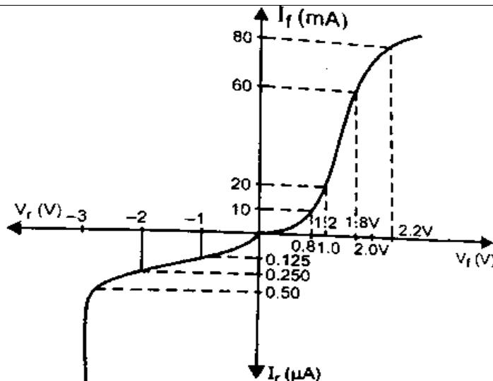
(i) Calculate the resistance of the diode during forward and reverse biasing.
