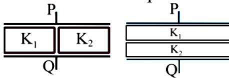
Ans Capacitance without a dielectric medium in between the plates  $C_0 = \frac{\epsilon_0 A}{d}$
