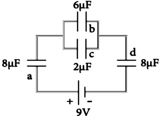
(a) Find the total capacitance of the given combination of capacitors.
