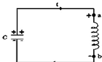
We know that a capacitor and an inductor can store electrical and magnetic energy, respectively. When a capacitor (initially charged) is connected to an inductor, the charge on the capacitor and the current in the circuit exhibit the phenomenon of electrical oscillations.
