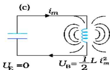
As the current reaches its maximum value  $i_m$ , (at  $t = T/4$ ) as in Fig.(c), all the energy is stored in the magnetic field:  $U_B = \frac{1}{2} L i_m^2$ . We can easily check that the maximum electrical energy equals the maximum magnetic energy. The capacitor now has no charge and hence no energy.
