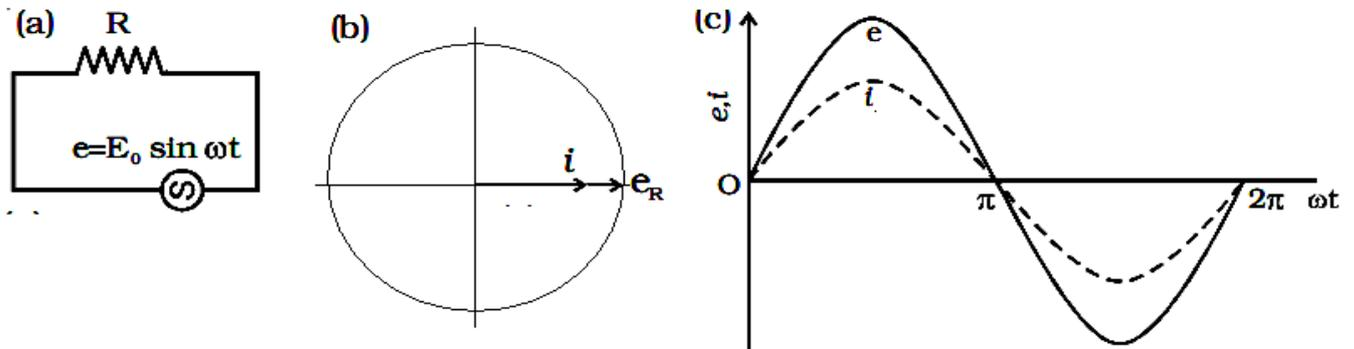
Let an alternating source of emf  $e = E_0 \sin \omega t$  be connected across a resistor of resistance  $R$ .
