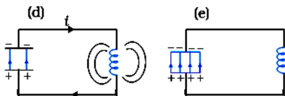
The current now starts charging the capacitor, as in Fig. (d). This process continues till the capacitor is fully charged (at  $t = T/2$ ) [Fig. (e)]. But it is charged with a polarity opposite to its initial state in Fig. (a).
