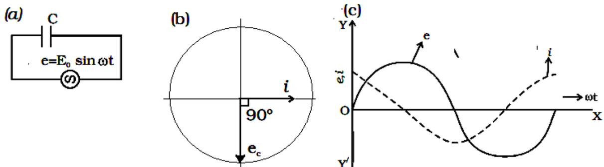
An alternating source of emf  $e = E_0 \sin \omega t$  is connected across a capacitor of capacitance  $C$ .
