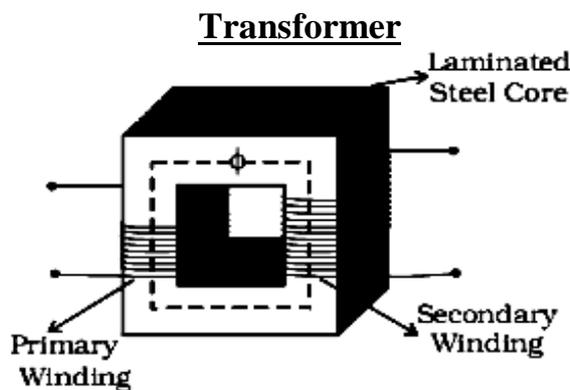
Transformer is an electrical device used for converting low alternating voltage into high alternating voltage and vice versa and transferring electric power from one circuit to another.
