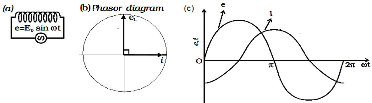
Let an alternating emf  $e = E_0 \sin \omega t$  be applied to a pure inductor of inductance  $L$ . Due to self induction of the coil , a self induced emf is generated which opposes the applied voltage..
