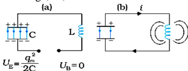
At  $t = 0$ , the switch is closed and the capacitor starts to discharge [Fig.(b)]. As the current increases, it sets up a magnetic field in the inductor and thereby, some
