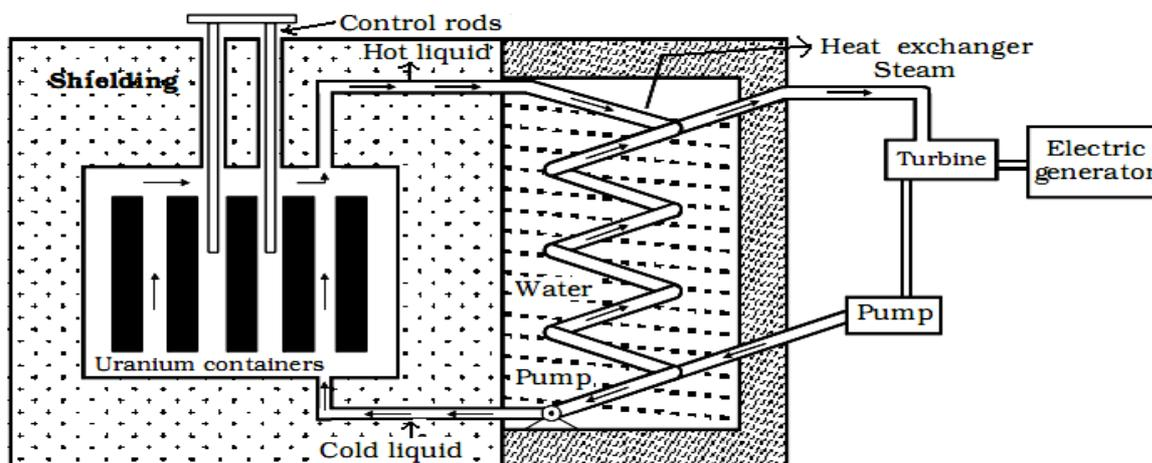
**(iii) Control rods:-**The control rods are used to control the chain reaction. They are very good absorbers of neutrons. They are made up of boron or cadmium. The control rods are inserted into the core and they pass through the space in between the fuel tubes and through the moderator. By pushing them in or pulling out, the reaction rate can be controlled. In our country, all the power reactors use boron carbide ( $B_4C$ ), a ceramic material as control rod.
